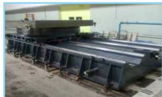
PERFORMANCE TESTING CNC ROTARY TABLE (40 Ton)
